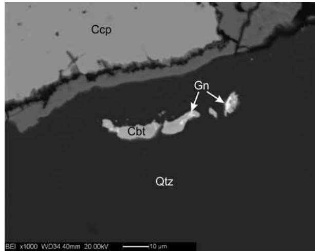
Fig. 27. Tiny grains of cobaltite (Cbt) and galena (Gn) in quartz (Qtz) close to chalcopyrite (Ccp) with an alteration vein at the quartz-chalcopyrite boundary.
